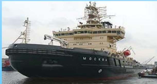
3. 16MW icebreaker for non-arctic waters
