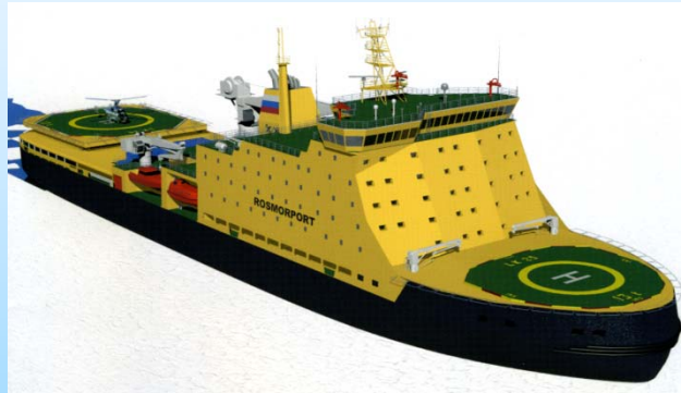
2. 25MW Diesel-powered icebreaker
