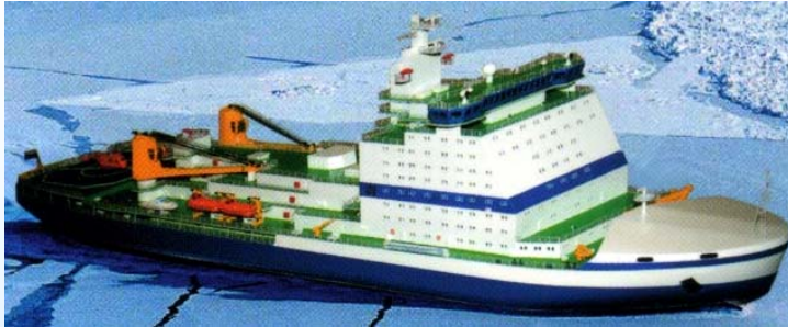
1. Multipurpose 60MW nuclear powered icebreaker (LK-60Ya)
